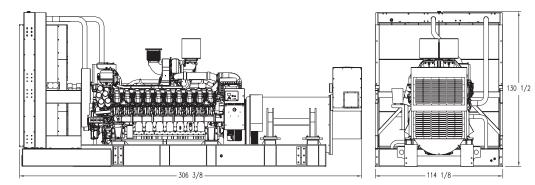
Drawing above for illustration purposes only, based on standard open power 480 volt generator. Lengths may vary with other voltages. Do not use for installation design.
